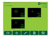
The <u>Power Window</u> provides access to all of the exhaust components controlled by the TruFlow. These include canopy lights, fan on/off, summer/winter and override settings.
