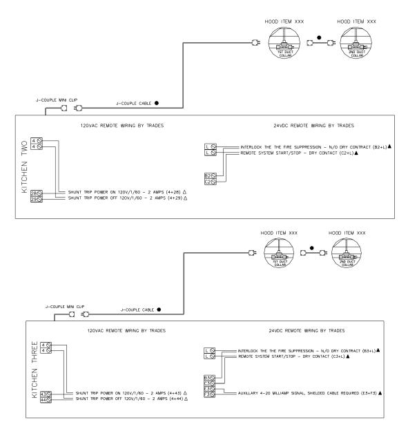
TRUFLOW Remote Control panel wiring schematic Three Kitchens
