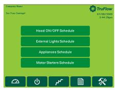
The automatic schedule is useful if you would like your exhaust system, external lights, appliances and motor starters to turn on and off at a set time each day. You can set up a different automatic start and stop time for each day of the week on each kitchen and motor starter. You will need to set an automatic start/stop time for every day of the week you will not be operating the exhaust system in manual (HAND) mode.
