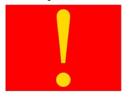
When an alarm that requires immediate attention or action occurs, the screen will change to red with a yellow exclamation mark. These types of alarm include certain drive errors where the VFD cannot reset automatically, and catastrophic equipment failures (exhaust fan or makeup air unit not running).
