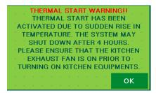
The TruFlow will automatically turn on the exhaust and supply fans when a threshold temperature under the hood is reached.
